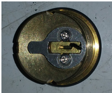
FIG 4) Remove the retainer
