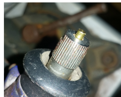
Fig 3) Screwdriver or other tool to take out retainer
