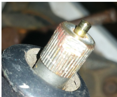
FIG 5) Put a pin in the dremel, trying to leave as much exposed as you can.
