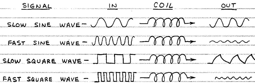
SOMETIMES A COIL WILL ADD RINGING TO A SQUARE WAVE PASSING THROUGH IT. THIS CAN HAPPEN WHEN THE RESISTANCE OF THE EXTERNAL CURRENT PATH THAT CONNECTS THE ENDS OF THE COIL IS HIGH.
