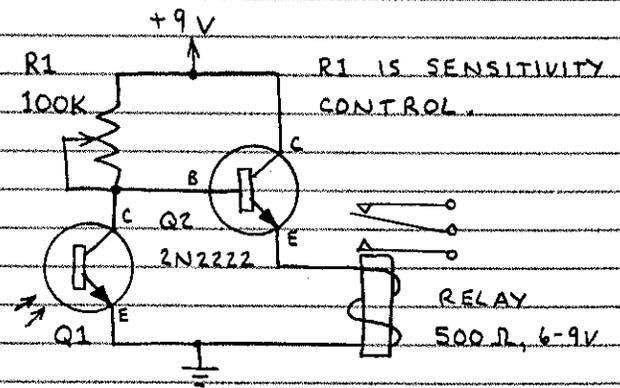
RELAY IS ACTUATED WHEN Q1 IS DARK. LIGHT ON Q1 DEACTUATES RELAY. CALIBRATE WITH R1.
