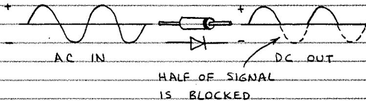
AN UNDULATING (AC) SIGNAL (OR VOLTAGE) IS RECTIFIED INTO A SINGLE POLARITY (DC) SIGNAL (OR VOLTAGE).
