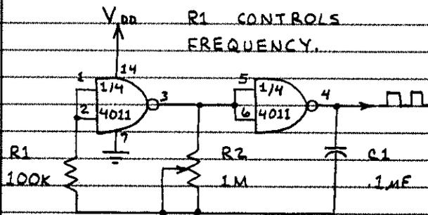
USE TO SUPPLY "CLOCK" PULSES TO OTHER CMOS CIRCUITS.
