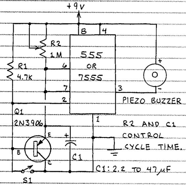
WHEN POWER IS APPLIED, THE 555 ENTERS A TIMING CYCLE. UNLESS S1 IS CLOSED BEFORE THE CYCLE ENDS, THE PIEZO BUZZER SOUNDS. THE CYCLE CAN BE RESET ANY TIME BY CLOSING S1. NOTE: S1 CAN BE REPLACED BY A SIGNAL FROM AN EXTERNAL CIRCUIT.
