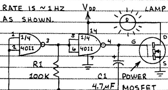
C1 AND R1 CONTROL RATE. OK TO USE SEPARATE SUPPLY FOR LAMP.
