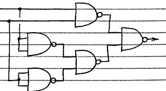
□ COMBINING DIFFERENT GATES — HERE ARE TWO EXAMPLES OF COMBINATIONAL NETWORKS THAT USE MORE THAN ONE KIND OF GATE. (REMEMBER, BOTH THESE CIRCUITS CAN ALSO BE MADE ENTIRELY FROM "NAND" GATES!)
