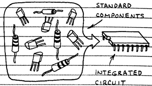
INTEGRATED CIRCUITS (OR IC'S) CAN CONTAIN AS FEW AS SEVERAL TO AS MANY AS HUNDREDS OF THOUSANDS OF TRANSISTORS. THEY HAVE MADE POSSIBLE VIDEO GAMES, DIGITAL WATCHES, AFFORDABLE COMPUTERS AND MANY OTHER VERY SOPHISTICATED PRODUCTS. HERE'S A SIMPLIFIED AND HIGHLY MAGNIFIED VIEW OF A SECTION OF A BIPOLAR INTEGRATED CIRCUIT:
