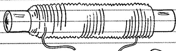
□ ELECTROMAGNET — INSERT A STEEL NAIL IN THE COIL, CONNECT THE LEADS TO A 9-VOLT BATTERY, AND THE NAIL WILL BECOME A MAGNET UNTIL THE POWER IS DISCONNECTED. (IT MAY RETAIN SOME MAGNETISM.)
