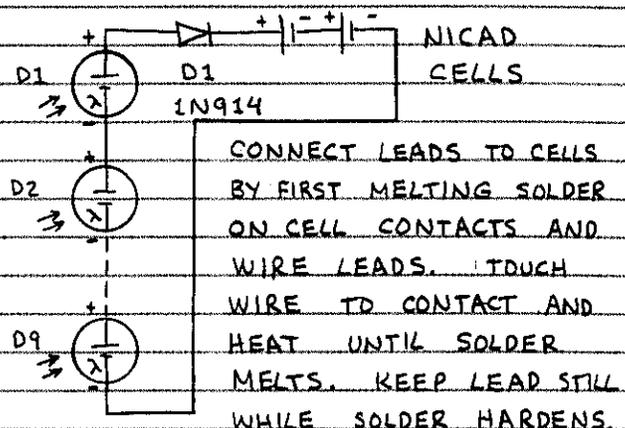
CONNECT LEADS TO CELLS BY FIRST MELTING SOLDER ON CELL CONTACTS AND WIRE LEADS. TOUCH WIRE TO CONTACT AND HEAT UNTIL SOLDER MELTS. KEEP LEAD STILL WHILE SOLDER HARDENS.
