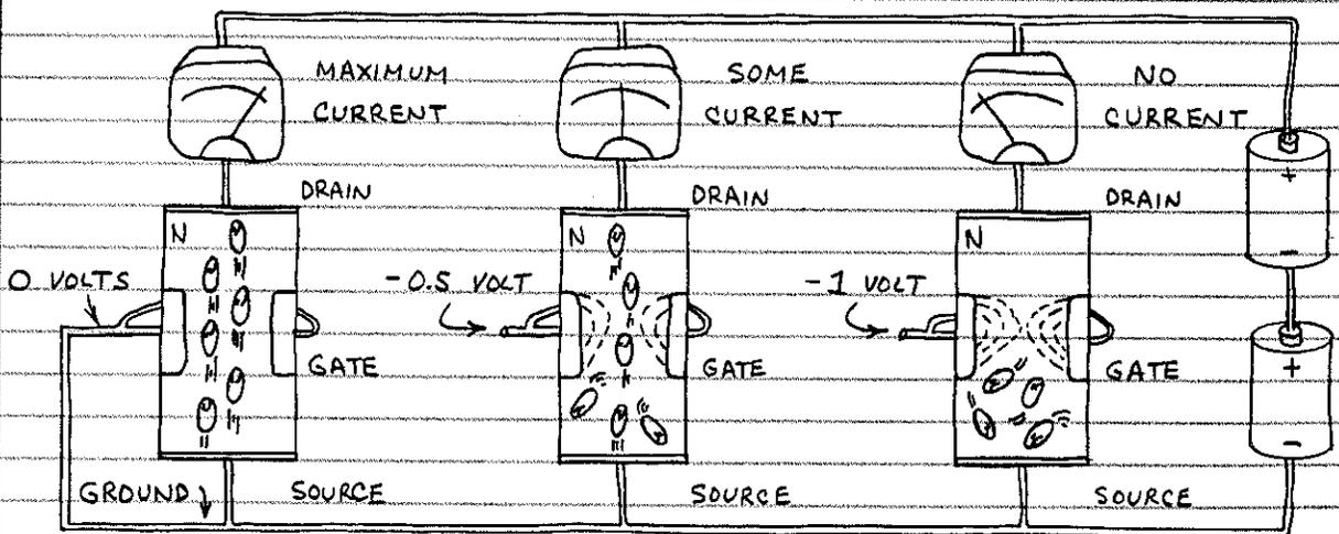
□ MORE ABOUT JUNCTION FETs — SINCE THEY ARE VOLTAGE CONTROLLED, JUNCTION FETs (OR JFETs) HAVE IMPORTANT ADVANTAGES OVER CURRENT-CONTROLLED BIPOLAR TRANSISTORS:
