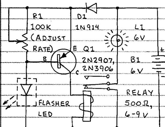
THE FLASHER LED INCLUDES A BUILT-IN IC THAT FLASHES THE LED SEVERAL TIMES EACH SECOND. THIS CIRCUIT SHOWS HOW TO "TAP" THIS FLASH RATE (VIA Q1) TO FORM AN ULTRA-SIMPLE PULSE GENERATOR THAT ACTUATES A RELAY AND, IN TURN, A LAMP. D1 IS NEEDED TO KEEP THE VOLTAGE TO THE FLASHER LED NEAR 5 VOLTS.
