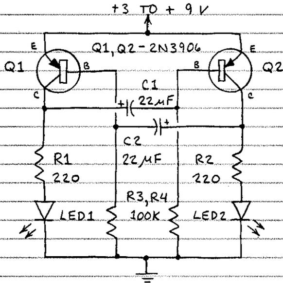
THIS CIRCUIT IS CALLED A FREE-RUNNING MULTIVIBRATOR. IT'S IDENTICAL TO A FLIP-FLOP THAT TRIGGERS ITSELF REPEATEDLY. Q1 AND Q2 ARE GENERAL PURPOSE PNP TRANSISTORS (2N3906, 2N2907, ETC.). R1 AND R2 LIMIT THE CURRENT TO THE LEDs (WHICH FLASH ALTERNATELY). INCREASING THE VALUES OF C1 AND C2 WILL SLOW THE FLASH RATE.
