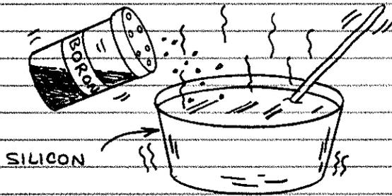
□ P & N SPICED SILICON LOAF — BORON, PHOSPHORUS AND CERTAIN OTHER ATOMS CAN JOIN WITH SILICON ATOMS TO FORM CRYSTALS. HERS'S THE CATCH: A BORON ATOM HAS ONLY THREE ELECTRONS IN ITS OUTER SHELL. AND A PHOSPHORUS ATOM HAS FIVE ELECTRONS IN ITS OUTER SHELL. SILICON WITH EXTRA PHOSPHORUS ELECTRONS IS CALLED N-TYPE SILICON (N=NEGATIVE). SILICON WITH ELECTRON DEFICIENT BORON ATOMS IS CALLED P-TYPE SILICON (P= POSITIVE).
