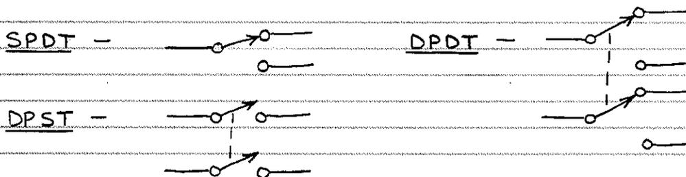
(THE DASHED LINE MEANS BOTH SIDES MOVE TOGETHER.)
