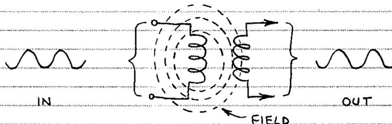
THE INPUT SIDE OF THE TRANSFORMER IS CALLED THE PRIMARY. THE OUTPUT SIDE IS CALLED THE SECONDARY.
