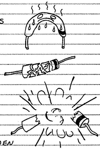
3. TOO MUCH REVERSE VOLTAGE WILL CAUSE A DIODE TO CONDUCT IN THE WRONG DIRECTION. SINCE THIS VOLTAGE IS FAIRLY HIGH, THE SUDDEN CURRENT SURGE MAY ZAP THE DIODE.
