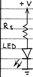
A SERIES RESISTOR MUST BE USED TO LIMIT CURRENT THROUGH AN LED. (EXCEPTIONS: CERTAIN PULSE CIRCUITS AND IC LED DRIVERS.)
