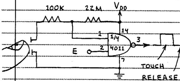
WHEN THE ENABLE INPUT (E) IS HIGH, THE CIRCUIT RESPONDS.
