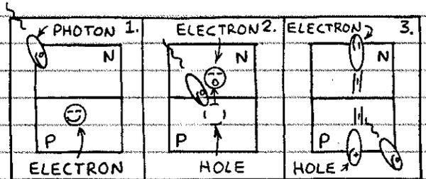
1. PHOTOVOLTAIC OPERATION - HERE THE PHOTODIODE BECOMES A CURRENT SOURCE WHEN IT IS ILLUMINATED.
