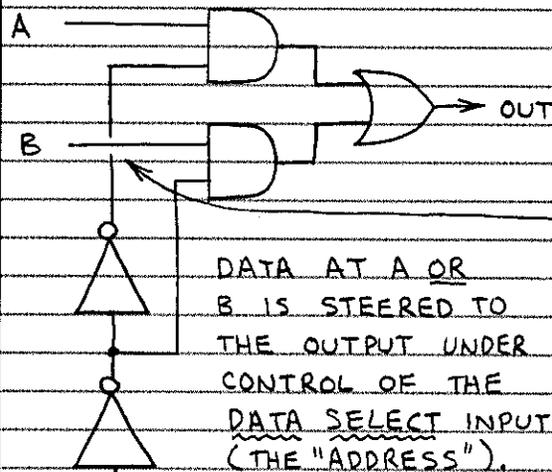
DATA AT A OR B IS STEERED TO THE OUTPUT UNDER CONTROL OF THE DATA SELECT INPUT (THE "ADDRESS").
