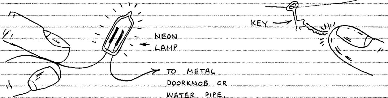
HERE'S A NEAT WAY TO "SEE" ELECTRICITY WITHOUT BEING ZAPPED! GRASP ONE LEAD FROM A NEON LAMP, WALK ACROSS A CARPET WHILE WEARING HARD SOLED SHOES AND TOUCH THE SECOND LEAD FROM THE LAMP TO A METAL OBJECT. THE LAMP WILL FLASH (UNLESS THE RELATIVE HUMIDITY IS HIGH).
