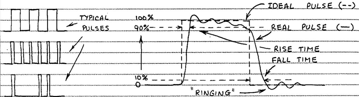
□ WAVES — A WAVE IS A PERIODIC FLUCTUATION IN A CURRENT OR VOLTAGE. WAVES MAY HAVE A SINGLE POLARITY (DC) OR BOTH POSITIVE AND NEGATIVE COMPONENTS (AC). THERE ARE MANY KINDS OF WAVES. HERE ARE A FEW:
