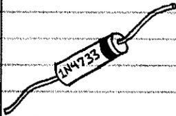
THE ZENER DIODE IS DESIGNED TO HAVE A SPECIFIC REVERSE BREAKDOWN (CONDUCTION) VOLTAGE. THIS MEANS ZENER DIODES CAN FUNCTION LIKE A VOLTAGE SENSITIVE SWITCH. ZENER DIODES HAVING BREAKDOWN VOLTAGES ( $V_z$ ) OF FROM ABOUT 2-VOLTS TO 200-VOLTS ARE AVAILABLE.
