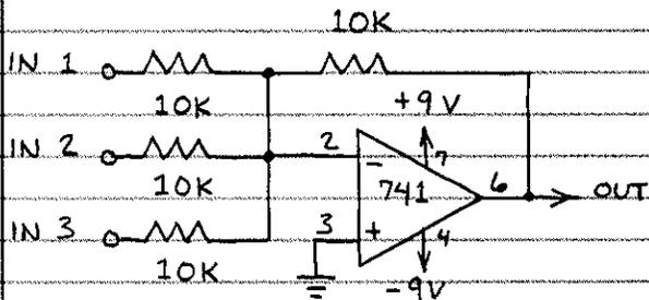
SEVERAL SIMULTANEOUS INPUTS. USE WITH AUDIO AMPLIFIER ABOVE.
