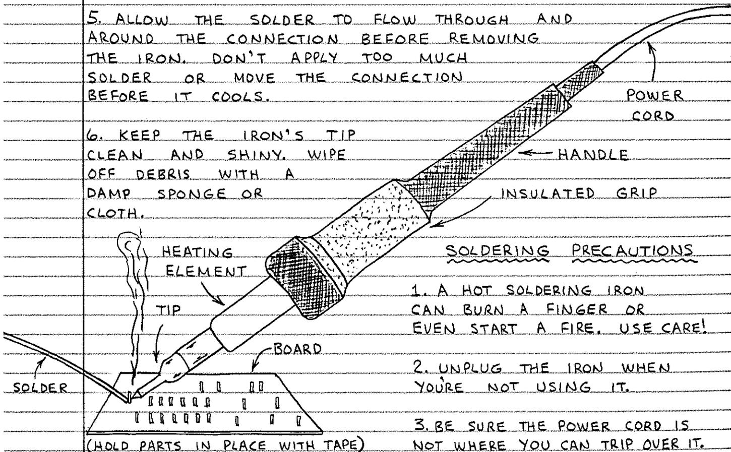
1. A HOT SOLDERING IRON CAN BURN A FINGER OR EVEN START A FIRE. USE CARE!
