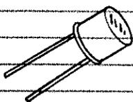
ALL DIODES RESPOND TO SOME DEGREE WHEN ILLUMINATED BY LIGHT. DIODES DESIGNED SPECIFICALLY TO DETECT LIGHT ARE CALLED PHOTODIODES. THEY INCLUDE A GLASS OR PLASTIC WINDOW THROUGH WHICH THE LIGHT ENTERS. OFTEN THEY HAVE A LARGE, EXPOSED JUNCTION REGION. SILICON MAKES GOOD PHOTODIODES.
