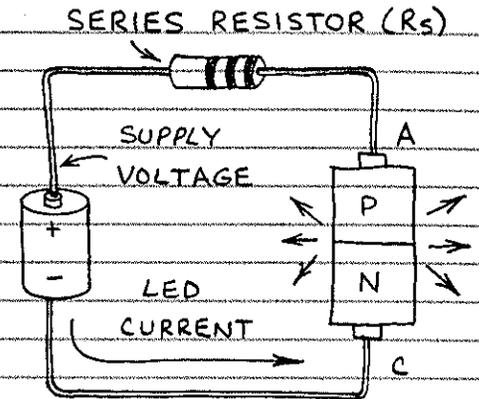
$$R_s = \frac{\text{SUPPLY VOLTAGE} - \text{LED VOLTAGE}}{\text{LED CURRENT}} \quad \text{OR} \quad R_s = \frac{V - V_{LED}}{I_{LED}} \quad \text{P.112}$$
