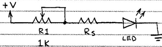
ADJUST  $R_1$  TO ALTER CURRENT THROUGH THE LED, THUS VARYING ITS BRIGHTNESS.  $R_s$  MUST BE USED (SEE ABOVE).
