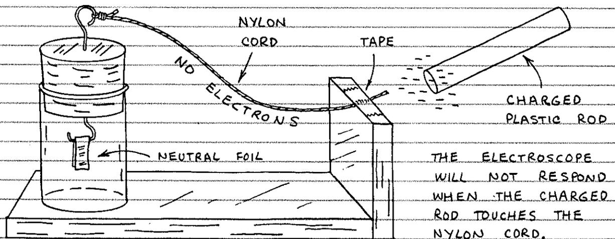
THIS DEMONSTRATION SHOWS THAT ELECTRONS CAN TRAVEL THROUGH SOME MATERIALS BUT NOT OTHERS. MATERIALS THROUGH WHICH ELECTRONS TRAVEL ARE CONDUCTORS. MATERIALS THROUGH WHICH ELECTRONS TRAVEL POORLY OR NOT AT ALL ARE INSULATORS.
