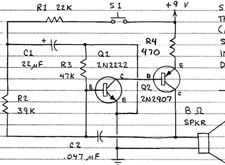
CLOSE S1 AND THE SPEAKER EMITS A TONE THAT RISES IN FREQUENCY (AS C1 CHARGES). OPEN S1 AND THE TONE FALLS IN FREQUENCY (AS C1 DISCHARGES). LIKE THIS:
