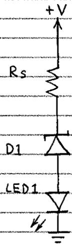
IN EACH CIRCUIT THE LED(S) GLOWS WHEN  $V+$  REACHES THE BREAKDOWN VOLTAGE ( $V_z$ ) OF ITS ZENER +  $V_{LED}$ . BE SURE TO USE INDIVIDUAL  $R_s$  FOR EACH LED. (SEE FACING PAGE.) THE CIRCUIT AT RIGHT PROVIDES A BAR-GRAPH READOUT WHEN ZENERS WITH PROGRESSIVELY HIGHER  $V_z$  ARE USED. CONNECT ZENERS IN SERIES FOR HIGHER TOTAL  $V_z$ .
