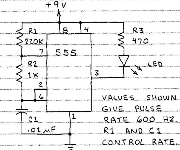
VALUES SHOWN GIVE PULSE RATE 600 HZ. R1 AND C1 CONTROL RATE.
