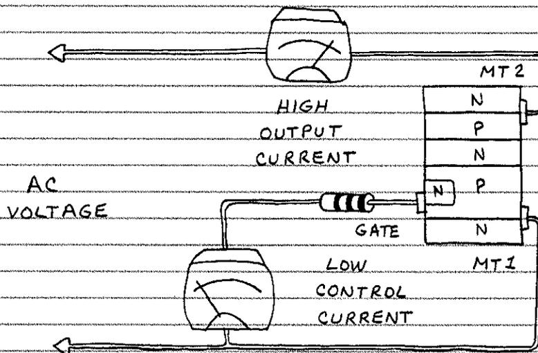
□ KINDS OF TRIACS — TRIACS, LIKE SCRS, ARE CATEGORIZED ACCORDING TO THE CURRENT THEY CAN SWITCH. TRIACS DON'T HAVE THE VERY HIGH POWER CAPABILITY OF HIGH CURRENT SCRS. HERE ARE TWO CATEGORIES:
