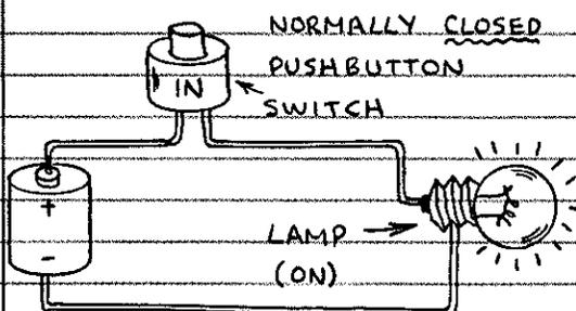
THE LAMP NORMALLY GLOWS. ONLY WHEN THE SWITCH IS OPENED IS THE LAMP OFF. IN OTHER WORDS, THE "NOT" GATE REVERSES (INVERTS) THE USUAL ACTION OF A SWITCH. HERE'S THE TRUTH TABLE:
