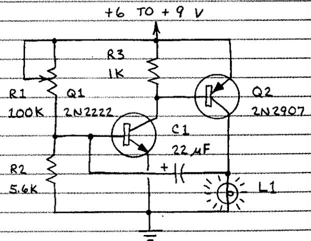
THIS CIRCUIT PRODUCES BRIGHT FLASHES EVERY SECOND OR SO. R1 CONTROLS FLASH RATE. USE NO. 122 OR 222 MINIATURE LAMP FOR L1.
