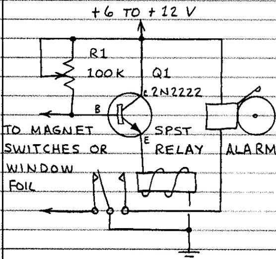
ALARM SOUNDS AND STAYS ON (UNTIL POWER IS DISCONNECTED) WHEN MAGNET SWITCH IS OPENED OR WINDOW FOIL IS BROKEN. R1: SET TO MAXIMUM VALUE. DISCONNECT ONE LEAD TO SWITCHES / FOIL. THEN REDUCE VALUE OF R1 TO JUST PAST POINT WHERE ALARM SOUNDS. CIRCUIT USES ONLY 0.3 MILLIAMPERES AT 6 VOLTS. RELAY: USE 6V, 500Ω UNIT WHEN SUPPLY IS 6-9 V. USE 12V, 1200Ω UNIT WHEN SUPPLY IS 12 V. NOTE: ASSEMBLE, INSTALL AND CONCEAL THIS SYSTEM WITH CARE.
