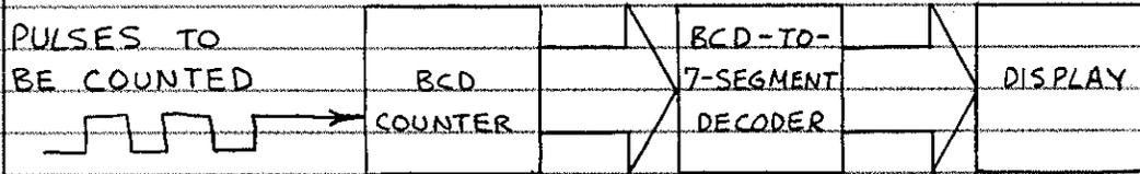
THE BCD COUNTER ADVANCES ONE COUNT FOR EACH INCOMING PULSE. WHEN THE COUNT REACHES 1001 (DECIMAL 9), THE COUNTER RECYCLES TO 0000. THE DECODER ACTIVATES THE APPROPRIATE SEGMENTS OF AN LED DISPLAY.
