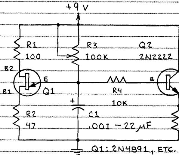
Q2 SAMPLES THE VOLTAGE ON C1 AND OUTPUTS IT AS A RAMP (OR "SAWTOOTH" WAVE). R3 CONTROLS THE RATE AT WHICH RAMPS ARE PRODUCED.
