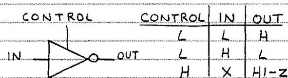
"X" MEANS "DOESN'T MATTER." HI-Z MEANS HIGH OUTPUT RESISTANCE.
