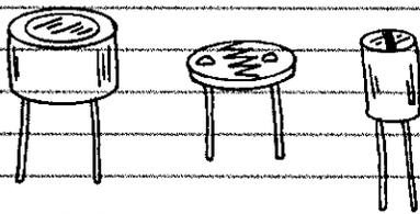
ARE AVAILABLE. IN MOST THE LIGHT SENSITIVE SEMICONDUCTOR IS COATED BETWEEN INTERLEAVED ELECTRODES TO INCREASE THE EXPOSED SURFACE. A PLASTIC OR GLASS WINDOW MAY OR MAY NOT BE USED.
