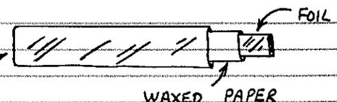
BE SURE THE FOIL SHEETS DON'T TOUCH! PRESS THE CONTACTS OF A 9-VOLT BATTERY BRIEFLY TO THE EXPOSED ENDS OF THE FOIL SHEETS. THEN TOUCH THE PROBES OF A HIGH-IMPEDANCE MULTIMETER TO THE FOIL SHEETS. THE METER WILL INDICATE A SMALL VOLTAGE FOR A FEW SECONDS. THE VOLTAGE WILL THEN FALL TO ZERO.
