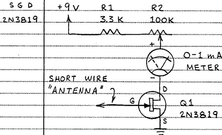
THIS CIRCUIT DETECTS STATIC ELECTRICITY FROM A CHARGED OBJECT (PLASTIC COMB, ETC.) OVER A FOOT AWAY! ADJUST R1 SO METER INDICATES 1 MA. CHARGED OBJECT NEAR "ANTENNA" WILL DECREASE METER READING.
