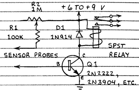
THIS CIRCUIT WILL MEASURE THE MOISTURE LEVEL OF SOIL IN YOUR GARDEN. ADJUST R2 FOR METER READING OF 1 mA WHEN SOIL MOISTURE IS AT DESIRED LEVEL. METER WILL THEN INDICATE LOWER MOISTURE LEVELS.
