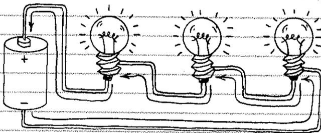
A CIRCUIT MAY INCLUDE MORE THAN ONE COMPONENT (SWITCH, LAMP, MOTOR, ETC.). A SERIES CIRCUIT IS FORMED WHEN CURRENT FLOWING THROUGH ONE COMPONENT FIRST FLOWS THROUGH ANOTHER. (ARROWS SHOW DIRECTION OF ELECTRON FLOW.)
