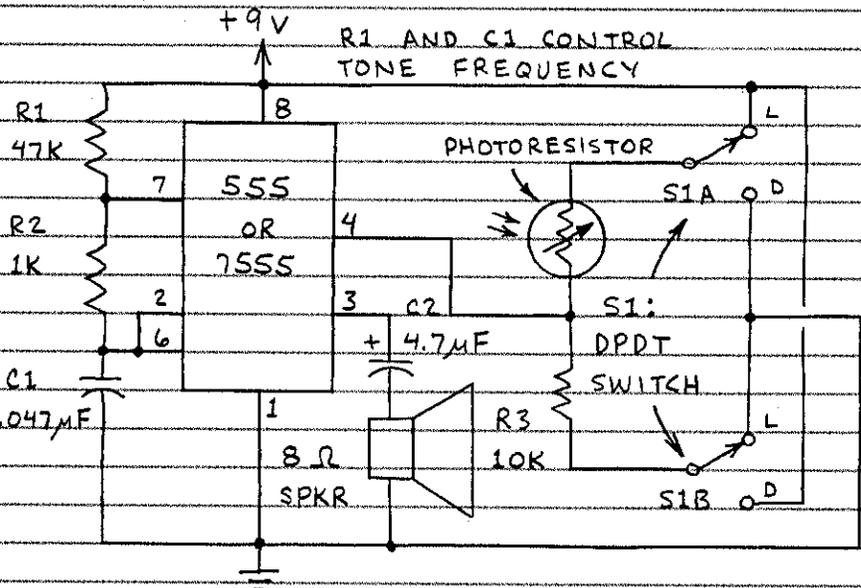
WHEN S1 IS IN POSITION "L," THE SPEAKER EMITS A TONE WHEN LIGHT ILLUMINATES THE PHOTORESISTOR. WHEN S1 IS IN POSITION "D," THE SPEAKER EMITS A TONE WHEN THE PHOTORESISTOR IS NOT ILLUMINATED.
