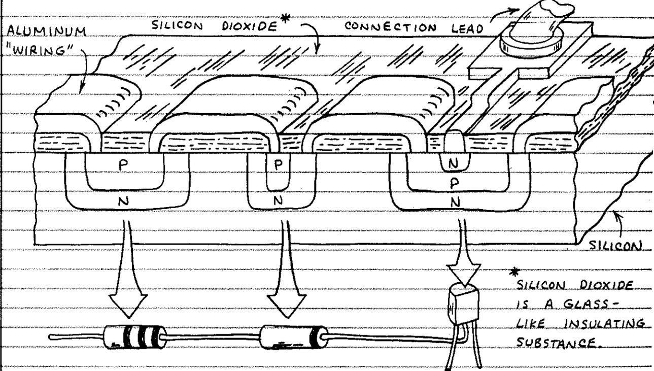
RESISTOR — A SMALL SECTION OF P-TYPE SILICON FORMS A RESISTOR.
