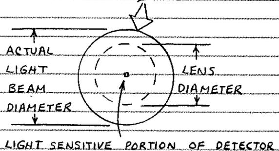
WITH CAREFUL LENS PLACEMENT ALL THE LIGHT WITHIN THE DASHED CIRCLE CAN BE FOCUSED ONTO THE LIGHT SENSITIVE PORTION OF THE DETECTOR. (SURE BEATS THE INVERSE SQUARE LAW!)
