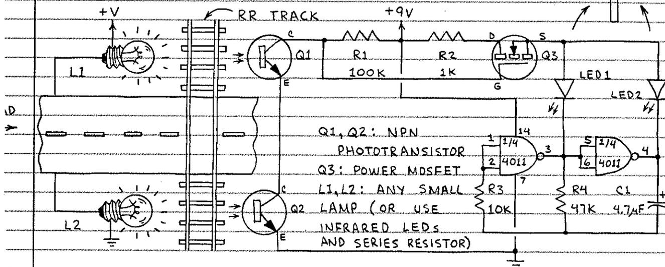
LEDs FLASH ALTERNATELY WHEN TRAIN BREAKS LIGHT BEAM TO EITHER Q1 OR Q2. LEDs CONTINUE FLASHING UNTIL TRAIN PASSES. SHIELD Q1 AND Q2 FROM ROOM LIGHTS WITH 1" HEAT SHRINK TUBING.
