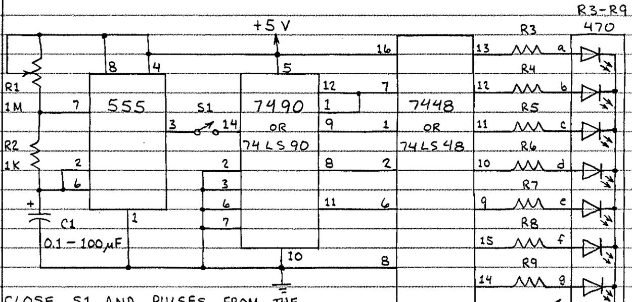
CLOSE S1 AND PULSES FROM THE 555 WILL BE COUNTED BY THE 7490. THE 7448 CONVERTS THE BCD OUTPUT FROM THE 7490 INTO 7-SEGMENT DIGITS ON AN LED DISPLAY. ADJUST R1 AND C1 FOR DESIRED PULSE RATE. TO ADD ADDITIONAL DIGIT:
