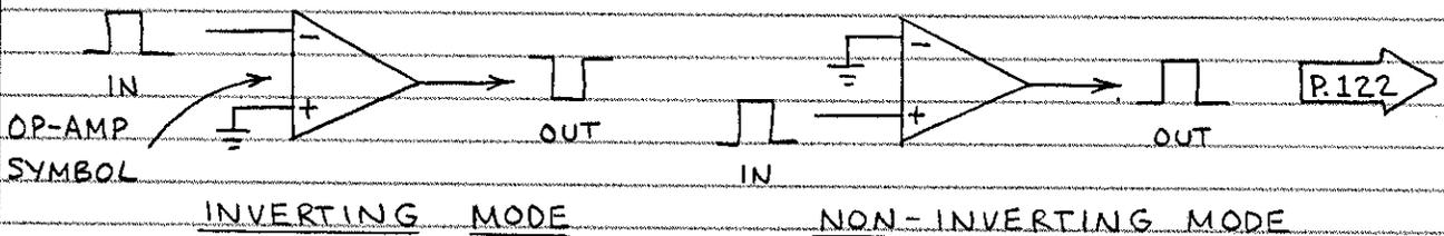
□ OP-AMP "FEEDBACK" — THE CIRCUITS SHOWN ABOVE ALLOW THE OP-AMP TO OPERATE AT ITS MAXIMUM AMPLIFICATION LEVEL (OR GAIN). USUALLY THE GAIN IS REDUCED TO A MORE PRACTICAL LEVEL BY FEEDING SOME OF THE OUTPUT BACK TO THE INVERTING (-) INPUT. FOR EXAMPLE:
