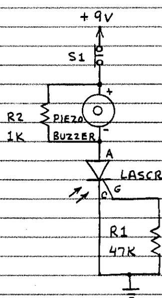
THESE CIRCUITS ARE ACTUATED BY LASCR LIGHT. OPEN S1 TO SWITCH LASCR OFF. SOME LASCRS ARE MORE LIGHT SENSITIVE THAN OTHERS. MOST WILL TRIGGER IN RESPONSE TO LIGHT FROM CAMERA STROBE (XENON FLASH UNIT).
