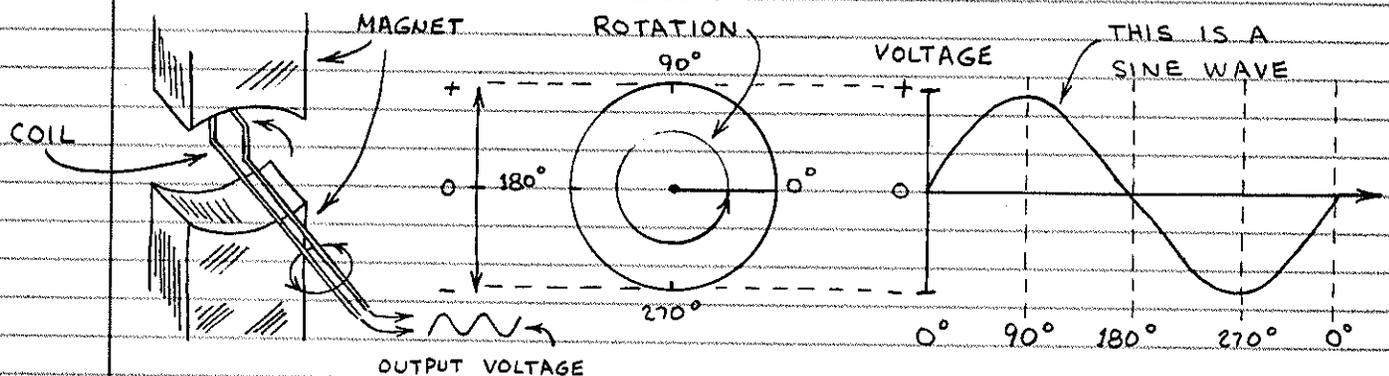
ROTATING COIL      VOLTAGE OUTPUT      AC SINE WAVE
