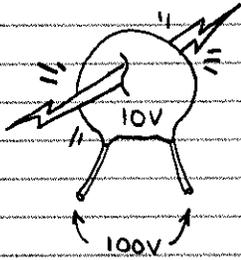
MAKE SURE THE CAPACITOR YOU PLAN TO USE MEETS OR EXCEEDS THE REQUIRED VOLTAGE RATING. OTHERWISE ITS DIELECTRIC MAY BE ZAPPED BY THE STORED CHARGE. THE VOLTAGE RATING IS USUALLY PRINTED ON THE CAPACITOR. V MEANS VOLTS. WV IS WORKING VOLTS (SAME THING).
