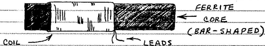
CHOKES. USED IN MANY CIRCUITS TO LIMIT OR SUPPRESS FLUCTUATING SIGNALS WHILE PASSING A STEADY CURRENT. CHOKES ARE AVAILABLE IN MANY SHAPES AND SIZES:
