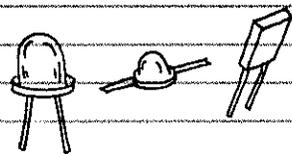
THESE INEXPENSIVE LEDs ARE USED AS INDICATOR LIGHTS. CERTAIN RED LEDs ARE USED TO TRANSMIT INFORMATION. MOST ARE ENCAPSULATED IN EPOXY.
