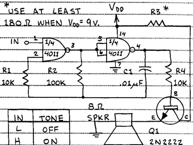
SENDS TONE TO NEARBY RADIO. TUNE RADIO AND/OR C1 TO HEAR TONE. USE INSULATED TOOL TO TUNE C1. C2 CONTROLS TONE FREQUENCY. USE 1-2 FEET OF WIRE FOR ANTENNA.
