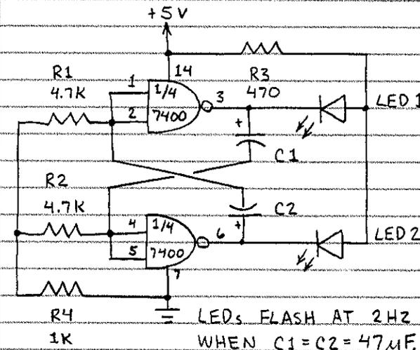
LEDs FLASH AT 2HZ WHEN C1 = C2 = 47μF
