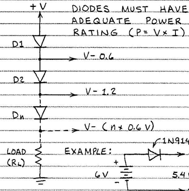
ONE OR MORE SILICON DIODES CAN REGULATE A VOLTAGE IN 0.6 VOLT STEPS.
