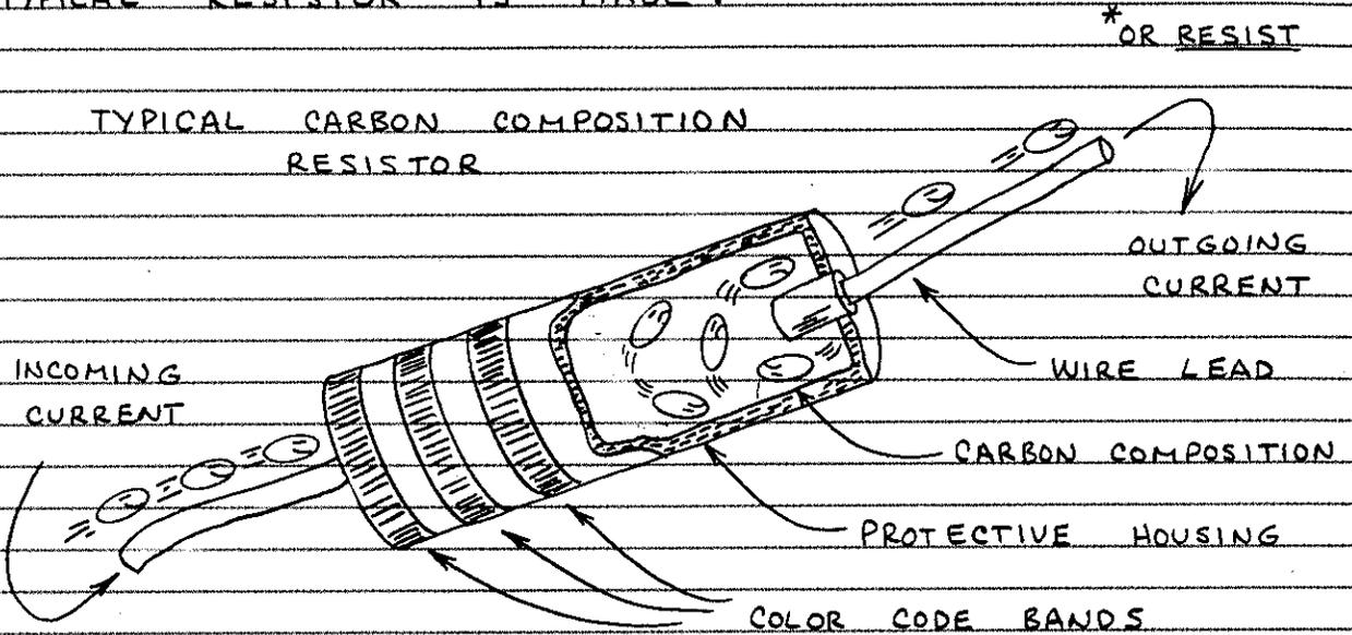
"CARBON COMPOSITION" IS JUST A FANCY WAY OF DESCRIBING POWDERED CARBON MIXED WITH A GLUE-LIKE BINDER. THIS KIND OF RESISTOR IS EASY TO MAKE. AND ITS RESISTANCE CAN BE CHANGED FROM ONE RESISTOR TO THE NEXT SIMPLY BY CHANGING THE RATIO OF CARBON PARTICLES TO BINDER. MORE CARBON GIVES LESS RESISTANCE.
