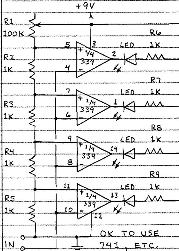
LEDs GLOW IN SEQUENCE AS INPUT VOLTAGE RISES. R1 CONTROLS SENSITIVITY.
