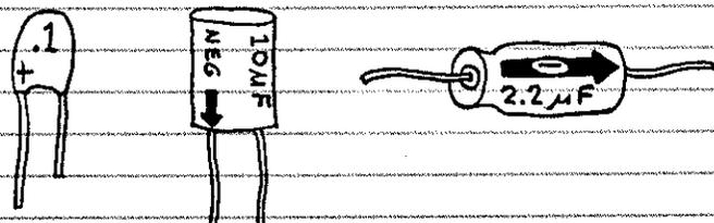
POSITIVE LEAD MUST GO TO MOST POSITIVE CONNECTION POINT!
