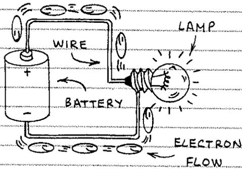
THIS BASIC CIRCUIT CONSISTS OF A SOURCE OF ELECTRICAL CURRENT (A BATTERY), A LAMP AND TWO CONNECTION WIRES. THE PART OF A CIRCUIT WHICH PERFORMS WORK IS CALLED THE LOAD. HERE THE LOAD IS THE LAMP. IN OTHER CIRCUITS THE LOAD CAN BE A MOTOR, A HEATING ELEMENT, AN ELECTROMAGNET, ETC.
