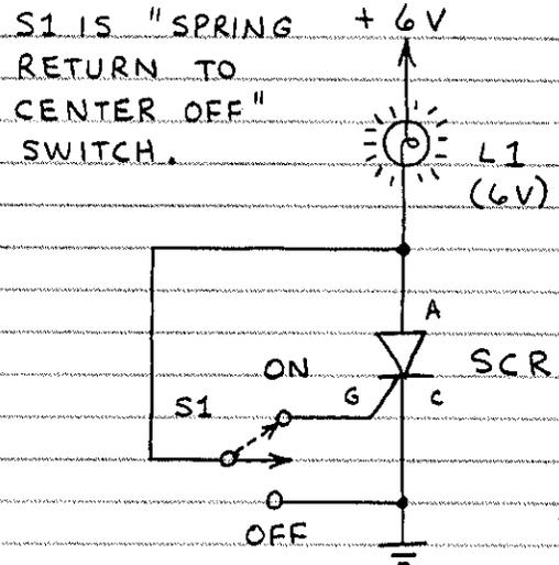
CLOSE S1 TO TURN ON THE SCR AND SUPPLY CURRENT TO THE LOAD. THE SCR WILL REMAIN ON AFTER S1 IS OPENED UNLESS THE LOAD IS A DC MOTOR OR UNTIL S2 IS BRIEFLY OPENED.
