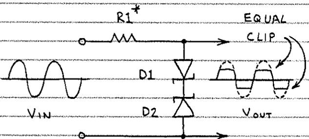
THIS IS A SYMMETRICAL FORM OF THE ADJACENT CIRCUIT. IT CLIPS BOTH HALVES OF AN INCOMING WAVE EQUALLY (IF  $V_z = D1 = D2$ ). USE TO PROTECT SPEAKERS AND PHONES FROM EXCESSIVE SIGNAL LEVELS OR TO MAKE SQUARE WAVES.
