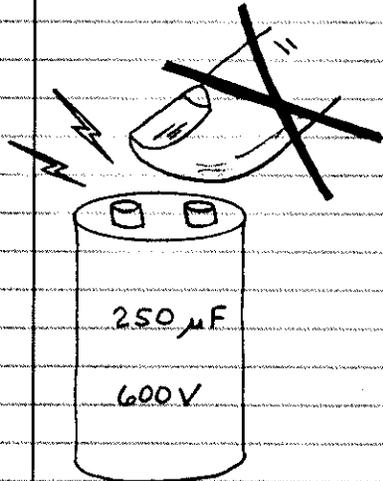
CAPACITORS CAN STORE A CHARGE FOR A CONSIDERABLE TIME AFTER THE POWER TO THEM HAS BEEN SWITCHED OFF. THIS CHARGE CAN BE DANGEROUS! A LARGE ELECTROLYTIC CHARGED TO ONLY 5 OR 10 VOLTS CAN MELT THE TIP OF A SCREWDRIVER PLACED ACROSS ITS TERMINALS! HIGH VOLTAGE CAPACITORS LIKE THOSE USED IN TELEVISION SETS AND PHOTOFLASH UNITS CAN STORE A LETHAL CHARGE! NEVER TOUCH THE LEADS OF SUCH A CAPACITOR. AT THE VERY LEAST THE JOLT CAN THROW YOU ACROSS A ROOM!
