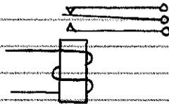
THIS IS THE SYMBOL FOR A RELAY WITH SPDT CONTACTS.
