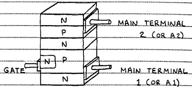
□ TRIAC OPERATION — THE TWO PARALLEL SCRS THAT FORM A TRIAC FACE IN OPPOSITE DIRECTIONS (REVERSE-PARALLEL). WHEN USED TO SWITCH ALTERNATING CURRENT, THE TRIAC STAYS ON ONLY WHEN THE GATE RECEIVES CURRENT. REMOVE THE GATE CURRENT AND IT SWITCHES OFF WHEN THE AC PASSES THROUGH 0 VOLTS.
