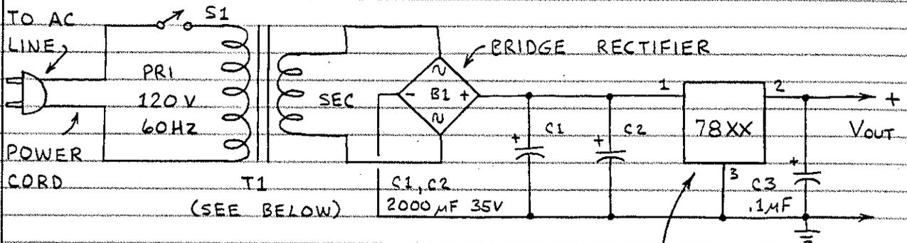
THIS BASIC SUPPLY WILL DELIVER UP TO 1.5 AMPERES AT THE RATED OUTPUT IF PROPERLY HEAT SUNK. YOU MUST USE A TRANSFORMER RATED AT THE PROPER VOLTAGE AND CURRENT. THE REGULATOR WILL "SHUT DOWN" IF THE CHIP BECOMES OVERHEATED. FOR BEST RESULTS APPLY SILICONE COMPOUND BETWEEN TAB AND HEAT SINK. ALL CONNECTIONS TO THE AC LINE MUST BE INSULATED OR ENCLOSED!
