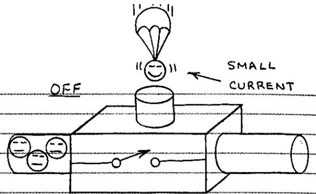
INSTEAD THEY ARE SOLID-STATE SWITCHES. THERE ARE TWO FAMILIES OF THYRISTORS, SILICON-CONTROLLED RECTIFIERS (SCRs) AND TRIACs. SCRs SWITCH DIRECT CURRENT AND TRIACs SWITCH ALTERNATING CURRENT.
