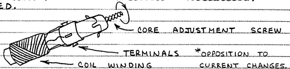
ANTENNA COIL. RADIOS OFTEN USE A BROADLY TUNED COIL TO PICK UP RADIO SIGNALS.
