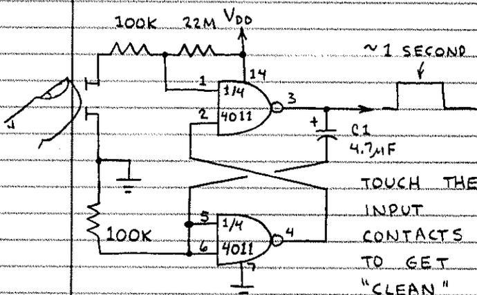
C1 CONTROLS LENGTH OF OUTPUT PULSE.
