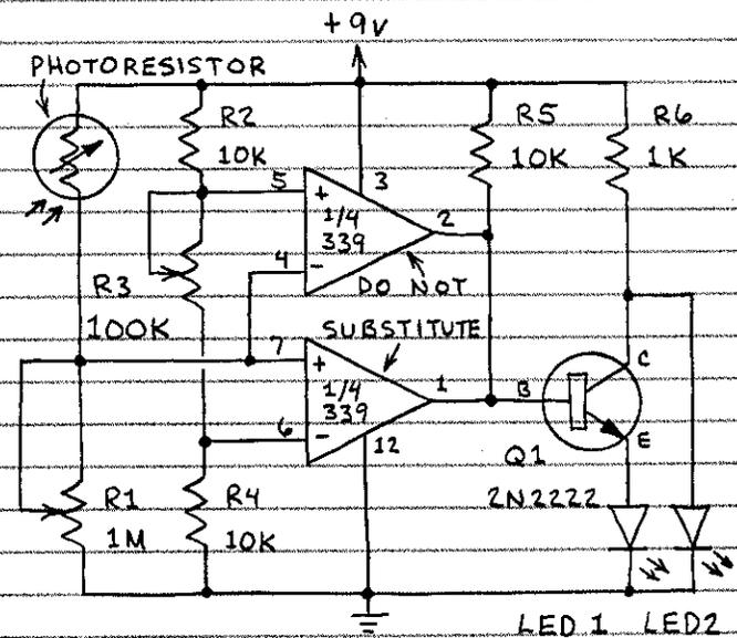
SET R1 TO CENTER POSITION. TURN OFF LIGHTS AND ROTATE R3 JUST PAST POINT WHERE LED 2 GLOWS. CIRCUIT WILL THEN RESPOND LIKE THIS: (R1 & R3 CONTROL RESPONSE)
