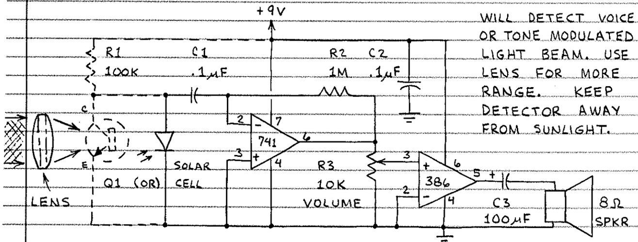
DETECTOR: USE R1 AND Q1 OR SOLAR CELL, (Q1: PHOTOTRANSISTOR)
