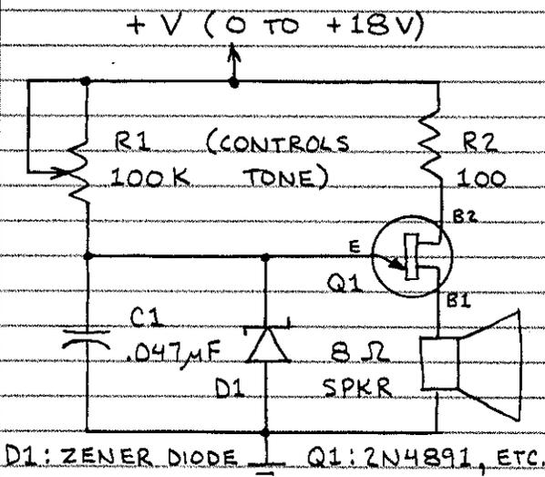
THIS CIRCUIT SOUNDS A TONE WHEN  $V_{IN}$  IS BELOW  $V_Z$  OF D1. SELECT  $V_Z$  OF D1 FOR DESIRED TURN-OFF LEVEL. THIS CIRCUIT CAN BE USED TO INDICATE WHEN VOLTAGE OF A BATTERY (WHICH CAN BE POWERING ANOTHER CIRCUIT) FALLS BELOW A CERTAIN LEVEL. THIS IS AN EXCELLENT EXAMPLE OF A SIMPLE, YET SOPHISTICATED, CIRCUIT.
