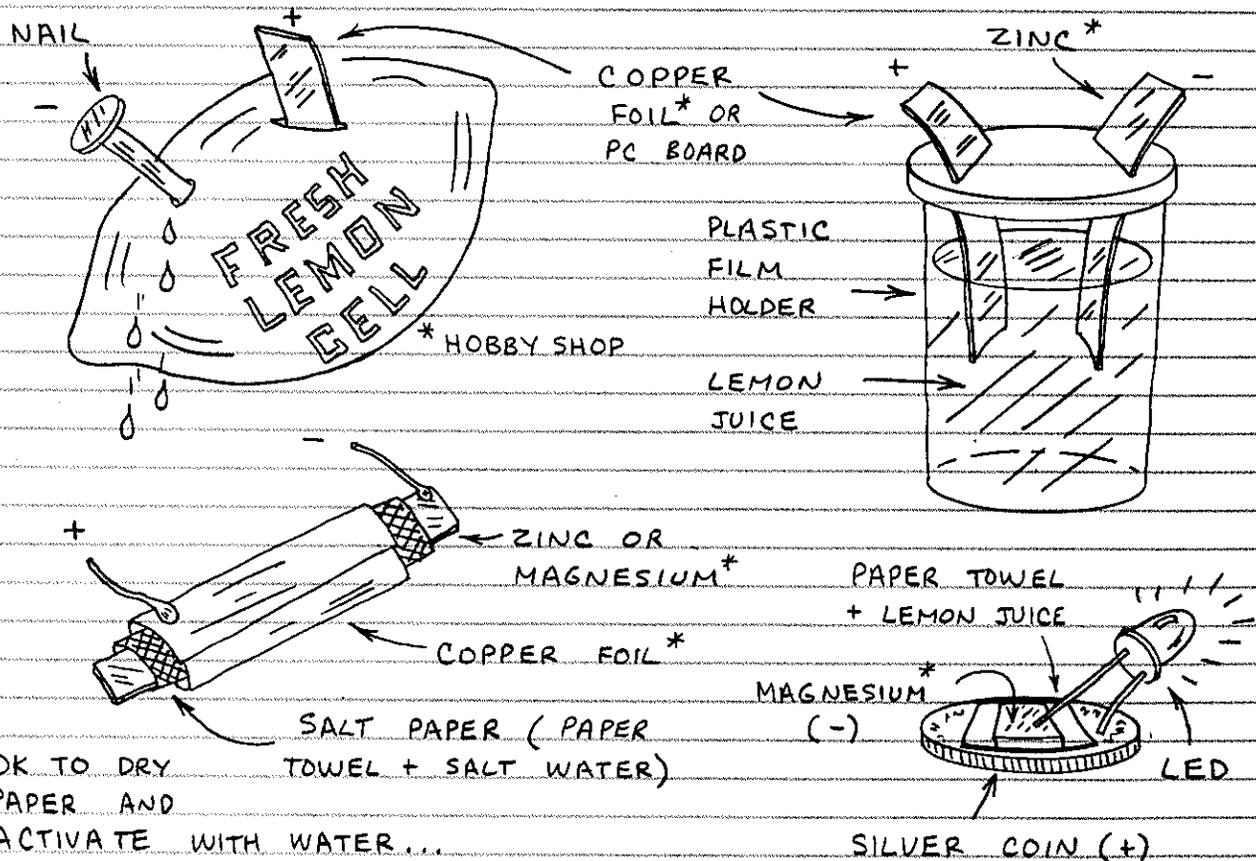
CONNECT TWO OR MORE CELLS IN SERIES TO FORM A BATTERY WITH TOTAL VOLTAGE EQUAL TO SUM OF CELL VOLTAGES.
