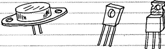
POWER TRANSISTORS ARE USED IN HIGH POWER AMPLIFIERS AND POWER SUPPLIES. LARGE SIZE AND EXPOSED METAL SURFACES KEEP THEM COOL.
