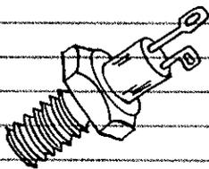
THESE SCRS CAN SWITCH UP TO 2,500- AMPERES AT UP TO SEVERAL THOUSAND VOLTS! THEY CONTROL MOTORS, LIGHTS, APPLIANCES, ETC.
