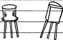
SMALL SIGNAL JFETs ARE USED AT THE INPUT STAGE OF AMPLIFIERS TO PROVIDE A HIGH RESISTANCE INPUT. THEY ARE ALSO USED AS SWITCHES.
