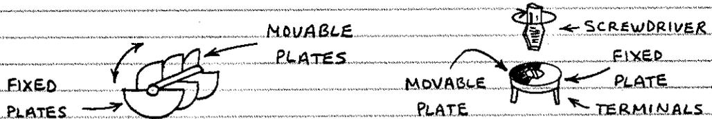
THIS KIND IS USED TO TUNE RADIO RECEIVERS AND TRANS-MITTERS. THE DIELECTRIC IS USUALLY AIR.
