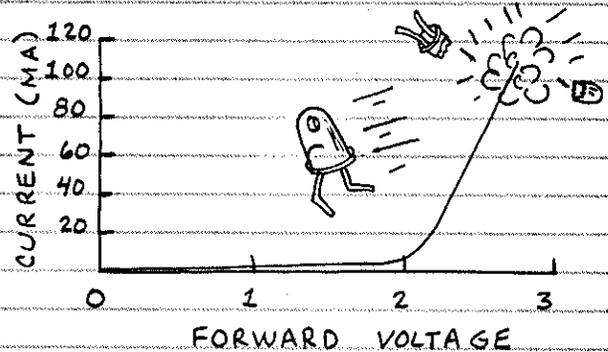
3. THE LIGHT EMITTED BY AN LED IS DIRECTLY PROPORTIONAL TO CURRENT THROUGH THE LED. THIS MEANS LEDs ARE IDEAL FOR TRANSMITTING INFORMATION. THE LIGHT OUTPUT FROM AN OVERHEATED LED WILL SOON DECREASE. THE LED MAY EVEN BE DAMAGED.
