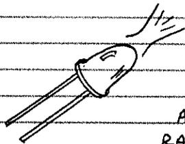
ALL DIODES EMIT SOME ELECTROMAGNETIC RADIATION WHEN FORWARD BIASED. DIODES MADE FROM CERTAIN SEMICONDUCTORS (LIKE GALLIUM ARSENIDE PHOSPHIDE) EMIT CONSIDERABLY MORE RADIATION THAN SILICON DIODES. THEY'RE CALLED LIGHT-EMITTING DIODES (LEDs).
