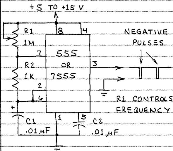
USE TO SUPPLY PULSES TO DIGITAL LOGIC CIRCUITS, ETC.
