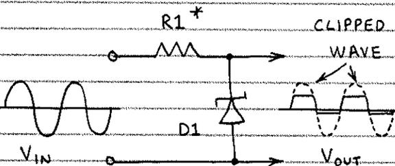
THIS CIRCUIT IS HANDY FOR REDUCING AN INCOMING SIGNAL VOLTAGE TO A LOWER, MORE MANAGEABLE LEVEL. IT CAN ALSO CONVERT A SINE OR TRIANGLE WAVE TO AN APPROXIMATION OF A SQUARE WAVE. \*R1: SEE ABOVE (LET  $I = 2$  MA MINIMUM).
