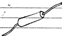
A DIAC IS A THREE-LAYER DEVICE SIMILAR TO A PNP JUNCTION TRANSISTOR WITHOUT A BASE LEAD. IT SWITCHES AC VOLTAGE.
