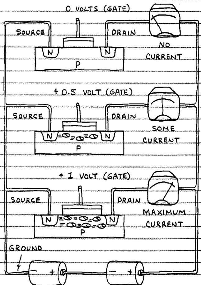
□ MORE ABOUT MOSFETS — THE INPUT RESISTANCE OF THE MOSFET IS THE HIGHEST OF ANY TRANSISTOR. THIS AND OTHER FACTORS GIVE MOSFETS IMPORTANT ADVANTAGES:
