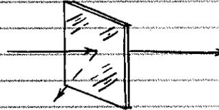
A GLASS MICROSCOPE SLIDE MAKES A GOOD BEAM SPLITTER. (EACH SURFACE REFLECTS 4%.)
