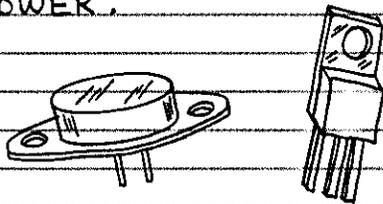
POWER MOSFETS ALLOW A FEW VOLTS TO SWITCH OR AMPLIFY MANY AMPERES AT VERY FAST SPEEDS.
